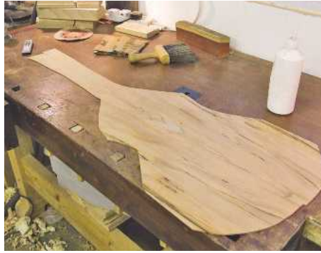
▲ Pic.2 Cut 3.5mm slices of padauk and sycamore for the top and bottom. Here you can see the sycamore book-matched for the top plate
